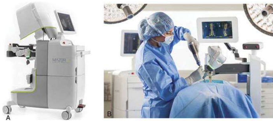
Figure 1.3: The Mazor X system: A) base station and robotic arm, B) bed and “patient”—mounted robotic arm.
